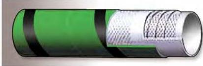
This suction and discharge hose, with its anti-static tube and conductive cover is excellent for wet or dry abrasive materials, like sugar or powdered milk. It's designed to be extremely flexible and suited for extreme environments.
