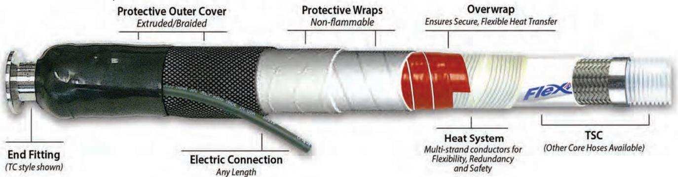
**EHH** is custom manufactured for a variety of applications to keep product flowing. Compared to single conductor heating elements, the **EHH** provides optimal heat transfer to a large (95%) surface area. Individual strand conductors are fixed in place and insulated with flexible, high-temperature fiber. The "Overwrap" layer of silicone rubber secures the conductors and provides a flexible cushion.
