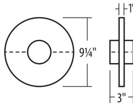
The Seal-Rite Hose Support provides additional protection for your transfer hoses. In environments where abnormal cover wear can occur, you can lift up and extend the life of your hose. The two halves easily attach with two recessed locking screws. The lightweight design, wide outer edges and even wider collar provides stability which eliminates kinking. Our supports are ideal for use in receiving bays to eliminate damming or pooling water.
