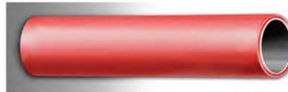
A rugged, abrasive and blister resistant hose for cleaning pumps, valves, tubing and equipment suitable for steam. Stands up to the harshest of environments with a specially formulated tube and cover that will not harden or crack during normal service. The steel braid reinforcement provides for safe use with steam pressures up to 250 PSI at 430° F.
