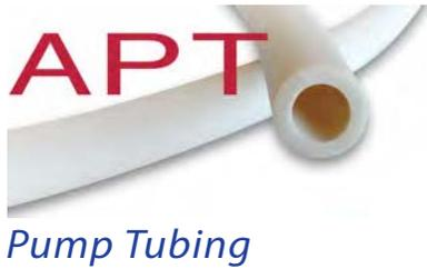
APT is ideal for pharmaceutical, biological, food and beverage applications and provides superior performance in peristaltic pumps. Extruded from virgin, medical grade TPR to precise dimensional tolerances and provides an excellent alternative to silicone tubing. APT is lot & batch traceable and can handle multiple autoclave cycles.
